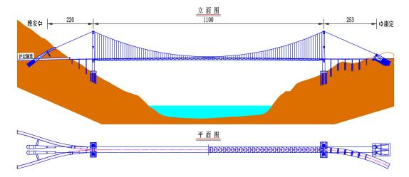
Fig. 3 Design and Elevation of Yakang Bridge
