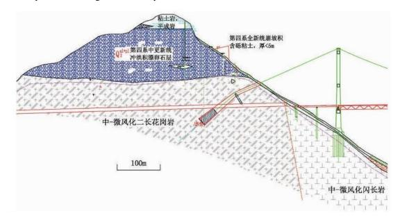
Fig. 5 Typical Engineering Geological Profile on the Left Bank (ChengQ, 2014)
