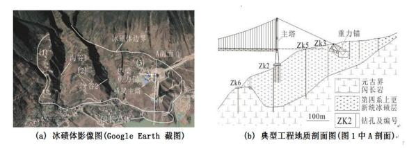
Fig. 7 Distribution characteristics of moraine soil layer (a) and the typical geological profile on the right
